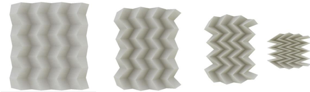
Figure 3: Various Deployable States of a Miura Pattern. Source: Computer Simulations Created Using FreeForm Origami (Tachi 2014)
