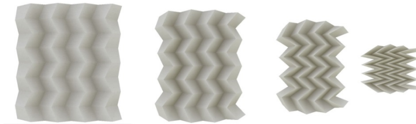
Figure 3: Various deployable states of a Miura pattern. Computer simulations created using FreeForm Origami by Tomohiro Tachi. Source: http://www.tsg.ne.jp/TT/software
