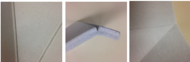
Figure 12. Cutting, scoring and folding of stiffened polyester felt panel.
